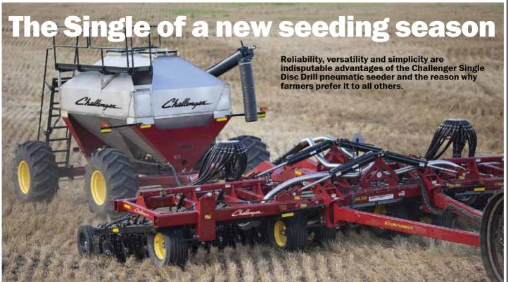
The special feature of this machine is the use of a patented technology of juxtaposed single discs which raise and remove the soil between 15 cm rows. The loosened soil is moved from the juxtaposed discs back to the roll-on wheel, which levels and compacts soil on the furrow. Such removal of the soil prevents the compacting of the lateral side and penetration of stubble into the furrow, thus contributing to regular sprouting.
