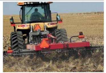
which one needs only to slightly slacken the battery bolts, set the required angle and then tighten the fastening bolts again. The multiple-purpose lifting system ensures a smooth penetration of tools into the soil and excellent tilling depth.
