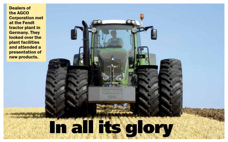
The guests beheld the upgraded Fendt 936 Vario tractor in all its glory. Plant engineers say that about 60 modifications were introduced in the previous model in order to make the machine more efficient and productive. Vario hydraulic and transmission systems were upgraded. New strengthened internal housing was installed in order to make service life of the hydraulic pump substantially
