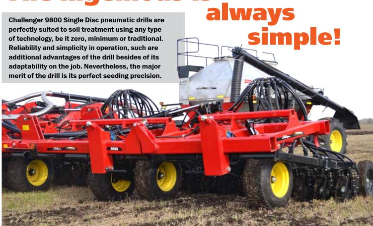
The secret of precise seeding is ingenious and simple. The key lies in design of the tool featuring the employment of opposed single discs that raise and move the soil between two 15 cm rows. The soil loosened by opposed discs is moved back to the roll-on wheel which levels and compacts the furrow soil. Such soil removal prevents compression of the side wall and keeps the furrow from cluttering with stubble, all of which promotes sprouting well.
