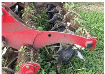
Vaederstad CrossCutter Disc is the new cultivator attachment developed especially for cutting and crushing rapeseed stubble immediately after the harvesting. Cultivation using this attachment encourages fallen seeds to germinate and decreases risks of fungus diseases and pest contamination.
