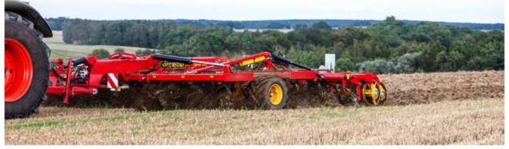
Opus is a versatile and unique cultivator which tills down to 40 cm (15 cm deeper than its legendary counterpart, the TopDown). With tines spaced at 27 cm and distributed across four axles, and with soil clearance of 80 cm, the cultivator can handle large amounts of after-harvesting residues while keeping the traction requirement moderate.
