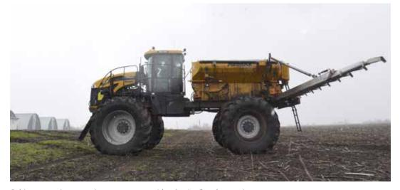
fluid pressure between the two spraying nozzles on the boom is 0.07 bars, which is outstanding for such equipment. Spray material is injected evenly. The durable steel boom is equipped with a stabilisation system for keeping the pre-set height even under difficult field conditions. AGCO Power, a low-consumption engine of the third generation equipped with a Common Rail fuel injection system, provides a good power margin. The sprayer starts up and gains required operating speed quickly.
