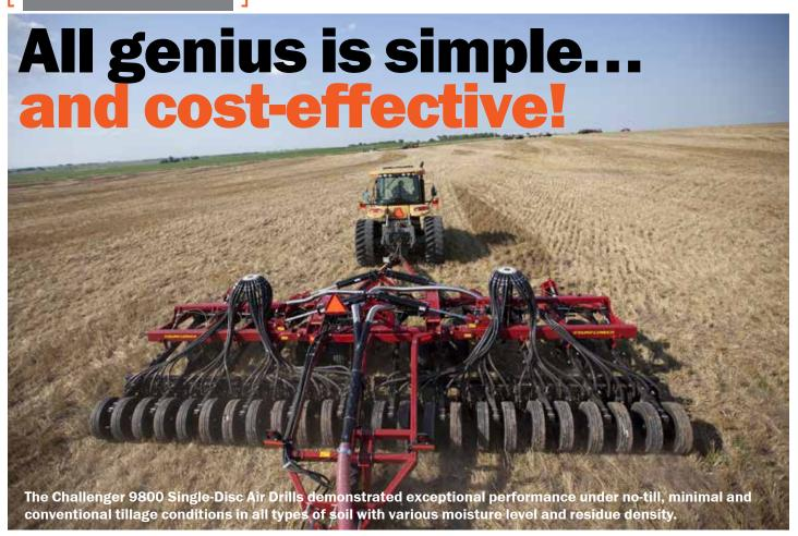
Farmers compare the young crops in the fields sown with the Single-Disc Drill to a smooth carpet. The simple design concept of Challenger — the opposing single discs — ensures perfect seed placement. The single-disc openers require less down pressure for soil penetration and form a sidewall without compaction.
