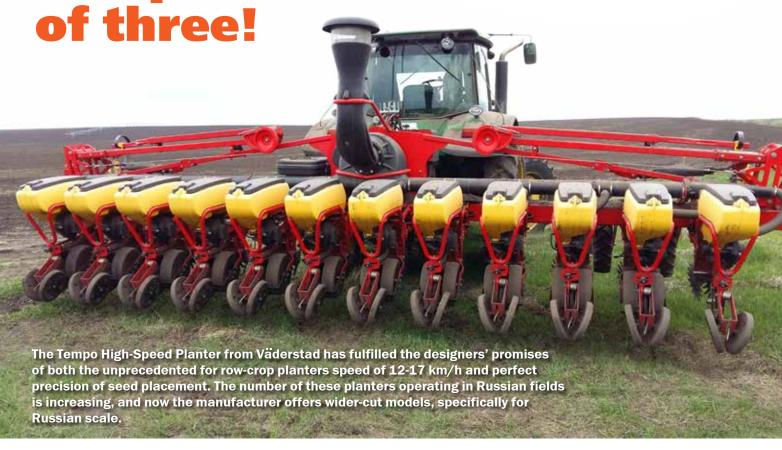
The brilliant PowerShoot solution of the Tempo drilling unit allows to plant faster without compromising the accuracy. The seed is 'shot' into the soil precisely at a set depth by pressurised air as compared to seed falling down to the soil through a pipe on most precision seed drills. Therefore, the vibration arising with the speed increase does not affect the quality and consistency of seed placement. Thus, traditional for sugar beets seeding rate of 5-8 km/h is no longer an issue.
