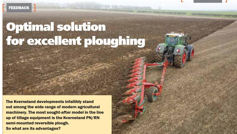
The manufacturer's hallmark is superior quality of metal. Due to the unique heat treatment technology (the frame is heat treated by induction twice and the temperature transfer to the steel is closely monitored), the plough frame gains triple strength while retaining lightness and flexibility. This directly affects the running cost of the plough: it requires less fuel and increases the service life of the tractor.
