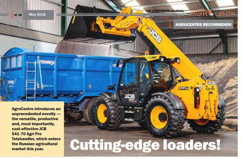
It is worth saying that this is the first telehandler in the world with the JCB DualTech VT hybrid transmission combining the advantages of hydro-mechanical and hydrostatic transmissions. The machine is designed to perform a number of different agricultural operations. The hydrostatic drive provides precise low-speed manoeuvring control, and the PowerShift drive guarantees superior high-speed efficiency and towing ability.
