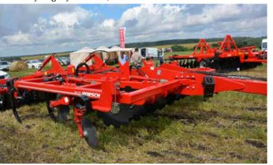
of AgroCentreLiski branch office in Oryol. 'The machine intensively crumbles heavy soils. Horsch Tiger 4 MT consists of a heavy two-row disc harrow and two rows of TerraGrip tines,
