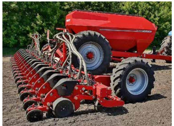
travel speed for precise seed placement is 8-12 km/h.' This year, Maestro 16 SW seed drills are going to show the precision they are capable of
