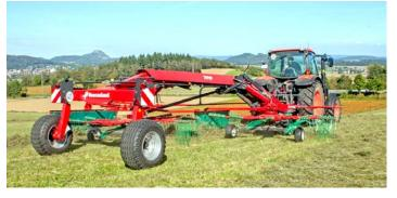
back, larger areas can be raked into one row. Both of the units can collect the green mass either into one large swath or two smaller ones, while the Kverneland 9670 S Vario provides even more flexibility as it can place two large swaths into one — with a total of up to 13.0 m of the green mass gathered into one swath.
